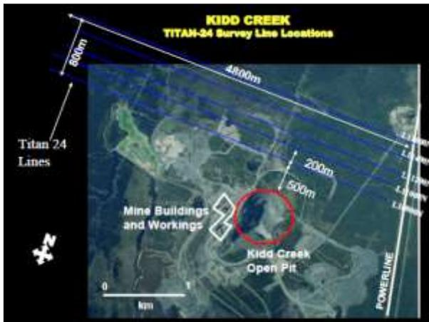
Figure 5. Survey lines near mine and power lines
