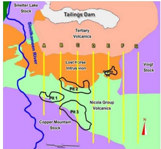
**Figure 3.** Copper Mountain Open pits and survey layout.
