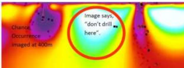
Figure 6 Resistivity section, shown to > 700m depth. Blue/ white regions represent resistive rock, warm colors represent increased conductivity
