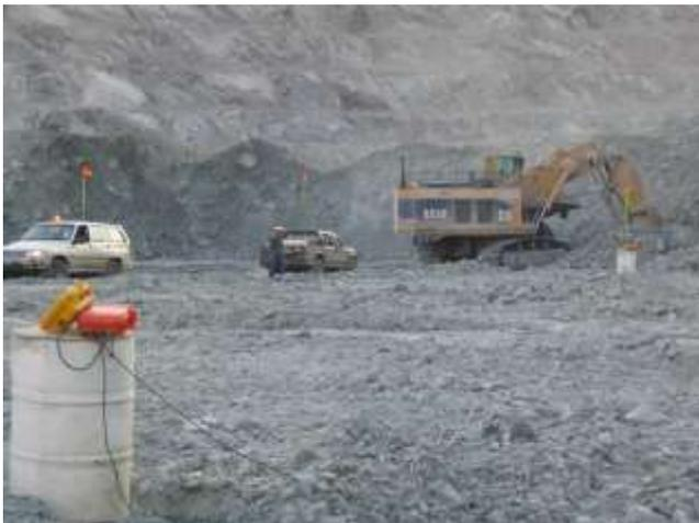
**Figure 2.** Deployment of deep imaging receivers in minesite.
