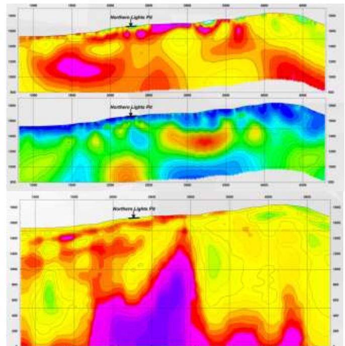
**Figure 1** (top) DC resistivity section from 2D TITAN24 distributed array survey. (middle) IP (chargeability) section I. Note how the DC model sees a near surface horizontal layer, senses a second deeper feature and senses something at the bottom of the section. (Bottom) The MT resistivity section corroborates the DC in the near surface but provides additional deeper imaging. Data courtesy Newmont, Nevada USA.
