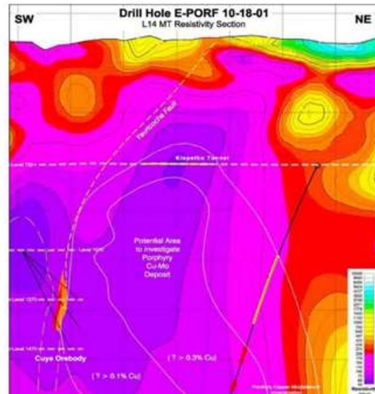
**Figure 10.** Deep MT resistivity with intersection at 1394 m.
