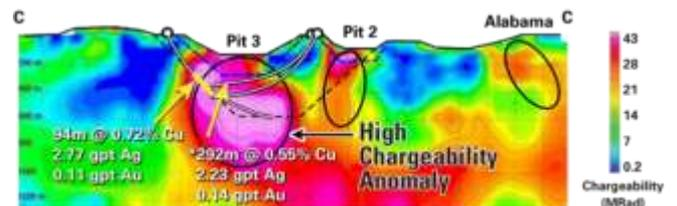
**Figure 4** Results from Line C. 2D chargeability section. The section is 750 meters deep and highlights new discoveries directly below existing open pits. Data courtesy Copper Mountain Mining, Canada.
