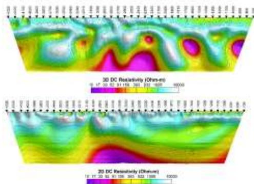
**Figure 9** Deep resistivity sections. Depth of the section is roughly 800 meters. (Top) 2D section sliced from a 3D inversion model of 3D data. (Bottom) 2D resistivity section from 2D inversion of single line of receivers. (2D data)
